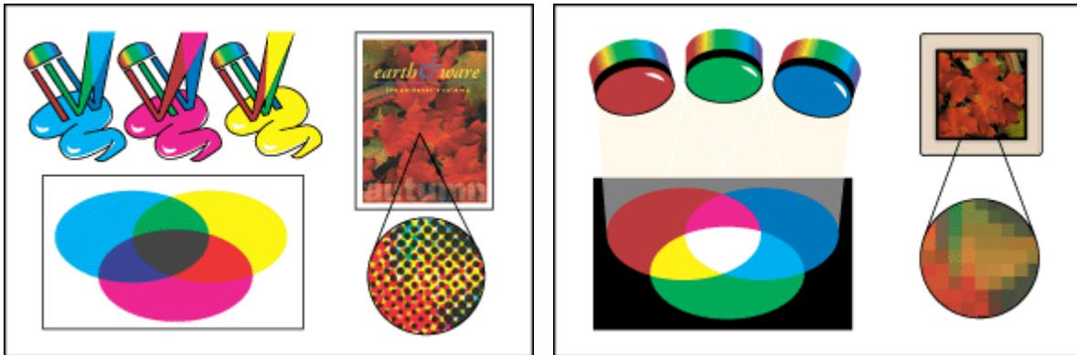
CMYK (left) and RGB color. Here you can see the dot pattern produced on a desktop printer vs. the pixels you will see on an RGB computer monitor (RGB printers produce dots, however).
